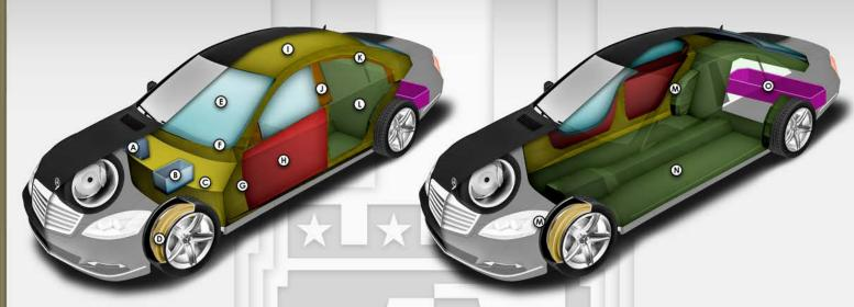
\*\* These schematics represent typical armoring of a sedan. The final vehicle (Mercedes-Benz S-Class) may vary depending on the client's required specifications. \*\*
