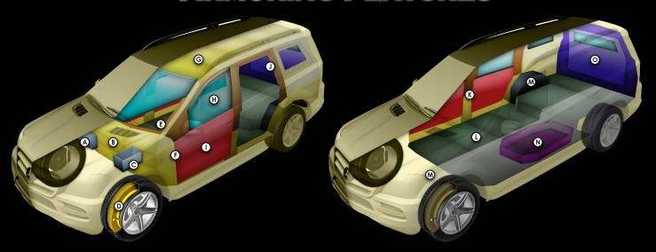
\*\* These schematics represent typical armoring of an SUV. The final vehicle (Cadillac Escalade ESV) may vary depending on the client's required specifications. \*\*
