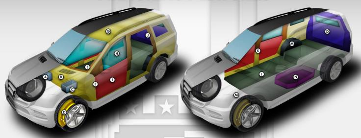
\*\* These schematics represent typical armoring of an SUV. The final vehicle (JEEP GRAND CHEROKEE SRT) may vary depending on the client's required specifications. \*\*
