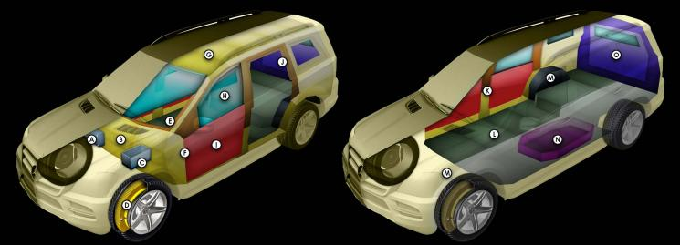
\*\* These schematics represent typical armoring of an SUV. The final vehicle (GMC Yukon Denali XL 4WD) may vary depending on the client's required specifications. \*\*
