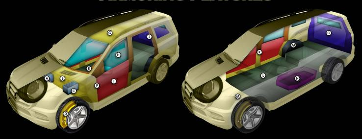
\*\* These schematics represent typical armoring of an SUV. The final vehicle (Cadillac Escalade ESV V-Series) may vary depending on the client's required specifications. \*\*
