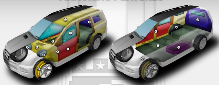
\*\* These schematics represent typical armoring of an SUV. The final vehicle (GMC Yukon Denali XL) may vary depending on the client's required specifications. \*\*
