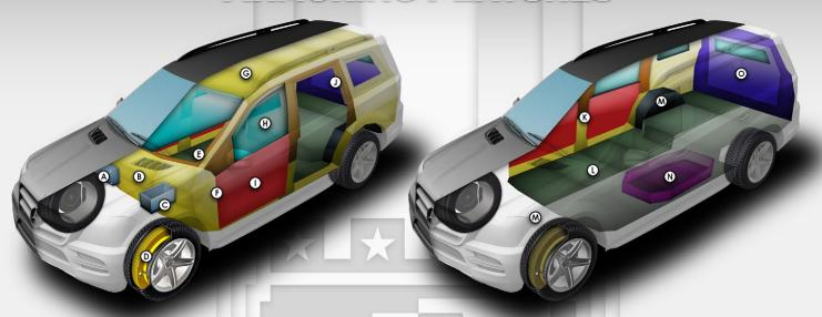
\*\* These schematics represent typical armoring of an SUV. The final vehicle (Ford Explorer Police - PPV) may vary depending on the client's required specifications. \*\*
