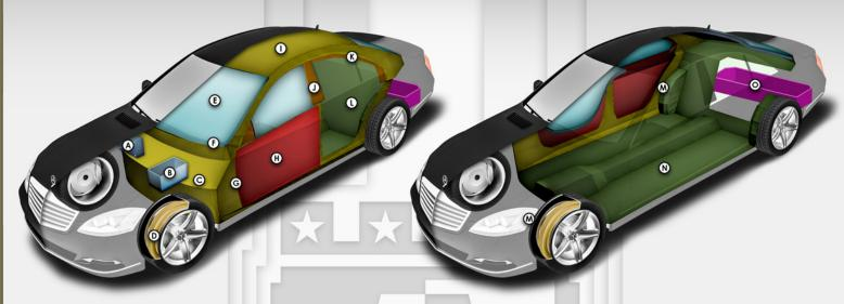
\*\* These schematics represent typical armoring of a sedan. The final vehicle (Mercedes-Benz \$550 4MATIC) may vary depending on the client's required specifications. \*\*
