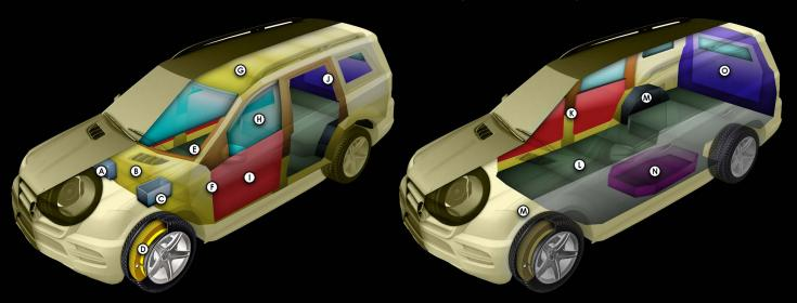
\*\* These schematics represent typical armoring of an SUV. The final vehicle (Lexus LX 600 Luxury) may vary depending on the client's required specifications. \*\*
