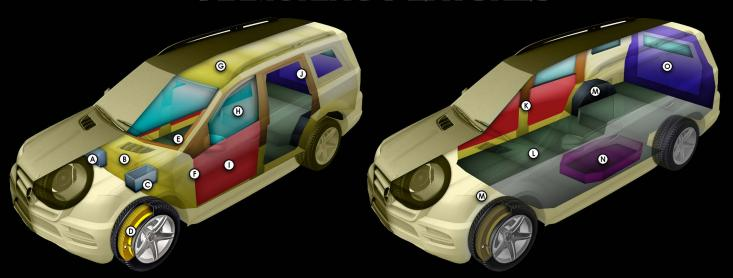
\*\* These schematics represent typical armoring of an SUV. The final vehicle (Toyota Seqouia Capstone) may vary depending on the client's required specifications. \*\*
