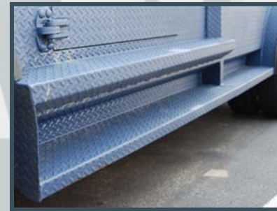
Exterior Running Boards Compliments the exterior grab handles, allowing personnel to ride on the outside
