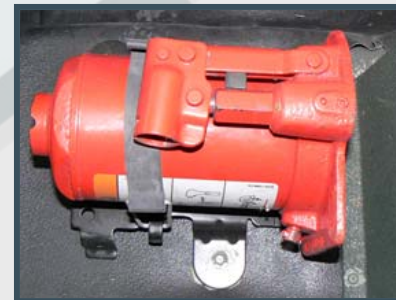
Heavy-Duty Jack Heavy-duty mechanical jack is included. Mounted behind front passenger seat
