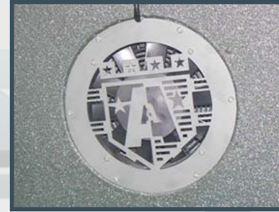
Air Flow Two exhaust fans are installed in the rear cabin to ensure optimal air flow
