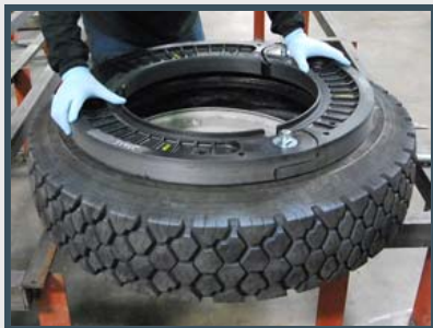
Run-Flat Inserts Six (6) run-flats installed
