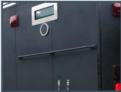
Exterior Grab Handle Rails Built-in exterior grab handles allow for quick arrival and deployment
