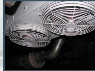
Air Flow Two exhaust fans are installed in the rear cabin to ensure optimal air flow
