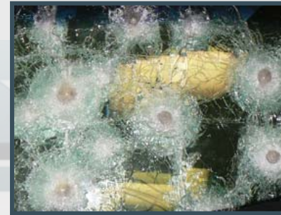
Glass Thickness 40 mm thick glass/polycarbonate
