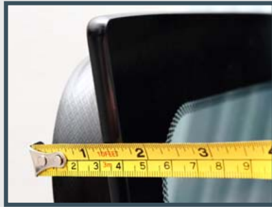
Glass Thickness 40 mm thick glass/polycarbonate
