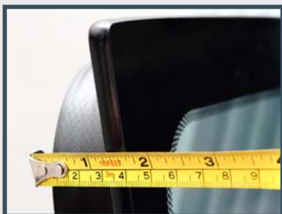
Glass Thickness 40 mm thick glass/polycarbonate
