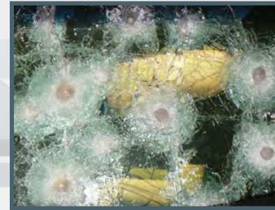
Window Thickness 55 mm thick glass/polycarbonate
