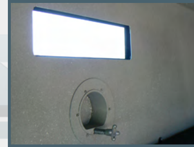
Rear Windows and Gun Ports Total of seven (7) viewing windows with dedicated gun ports under each (includes rear door)
