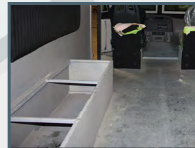
Rear Seating Storage Rear cabin features gear storage under each seat cushion
