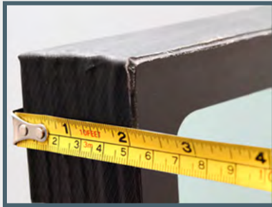
Window Thickness 55 mm thick glass/polycarbonate
