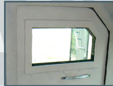
Layered Design Layered glass and composites protect against multiple hits, providing more time to escape
