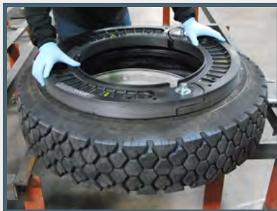
Run-Flat Inserts Six (6) run-flats installed
