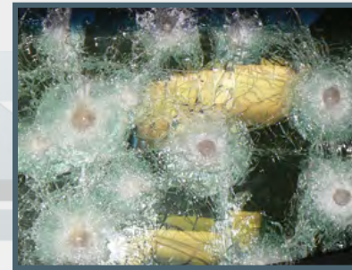
Multi-hit Protection 40 mm thick for maximum protection
