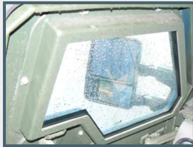
Window Thickness 40 mm thick glass/polycarbonate
