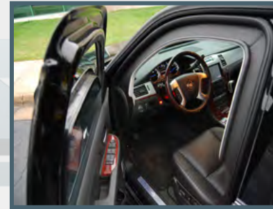
Window Thickness 40 mm thick for maximum protection
