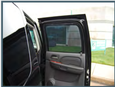
Anti-Spall Anti-spall layer prevents glass fragments from penetrating into passenger cabin
