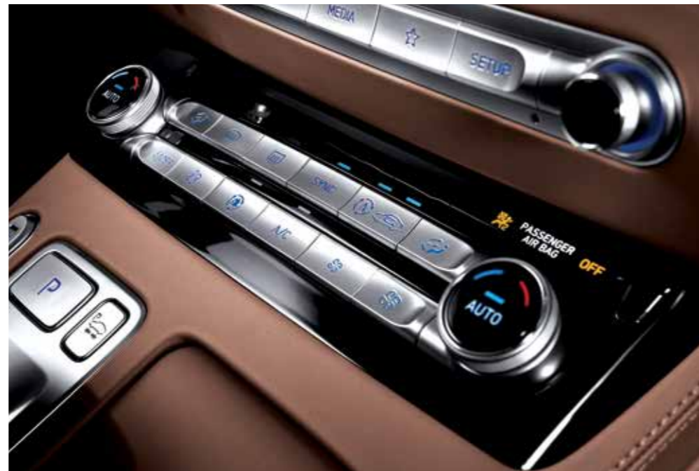
Chrome-plated buttons – The number of buttons on the center fascia has been dramatically reduced, and the remaining buttons are chrome-plated to make them both aesthetically pleasing and functionally convenient.
