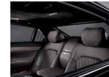
Automatically operated side curtains and rear windshield curtain for rear seats
