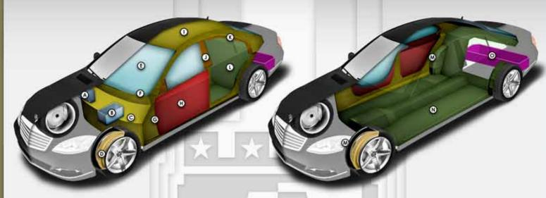
These schematics represent typical armoring of a sedan. The final vehicle (Lexus LS460 L) may vary depending on the client's required specifications. \*\*
