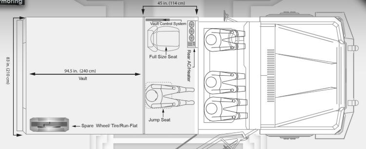
\*\* These schematics represent typical armoring of a truck. The final vehicle (Ford F-550 XL) may vary depending on the client's required specifications. \*\*
