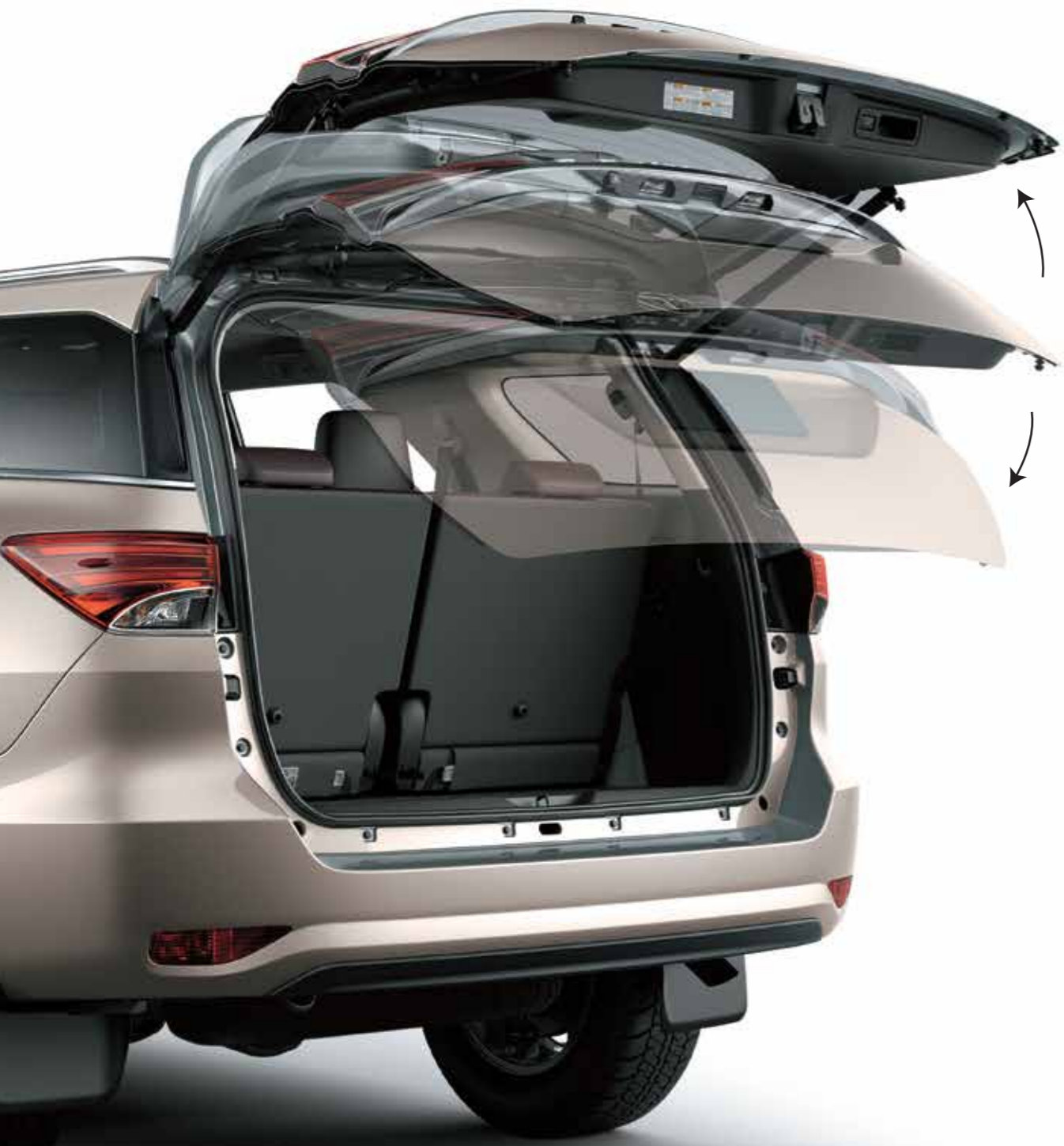
Electronically Controlled Power Back Door with Memory and Jam-Protection
