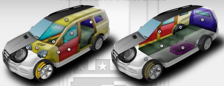
\*\* These schematics represent typical armoring of an SUV. The final vehicle (Chevrolet Silverado 1500) may vary depending on the client's required specifications. \*\*
