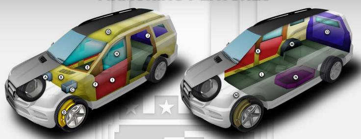
\*\* These schematics represent typical armoring of an SUV. The final vehicle (TOYOTA 4RUNNER TRD) may vary depending on the client's required specifications. \*\*
