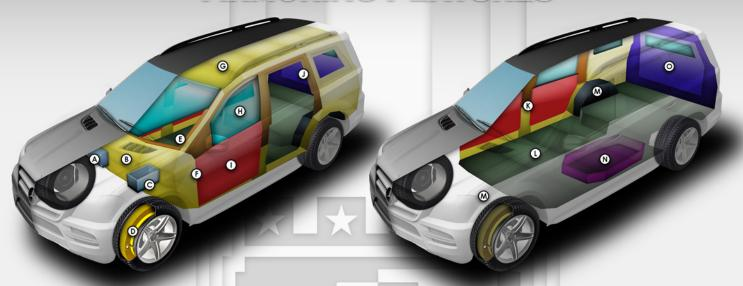
\*\* These schematics represent typical armoring of an SUV. The final vehicle (Chevrolet Tahoe High Country) may vary depending on the client's required specifications. \*\*
