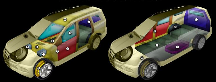
\*\* These schematics represent typical armoring of an SUV. The final vehicle (Omicron Land Cruiser 78) may vary depending on the client's required specifications. \*\*
