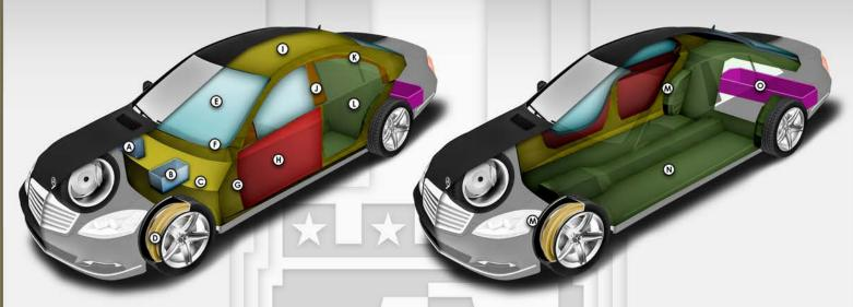
\*\* These schematics represent typical armoring of a sedan. The final vehicle (Mercedes-Benz S580) may vary depending on the client's required specifications. \*\*
