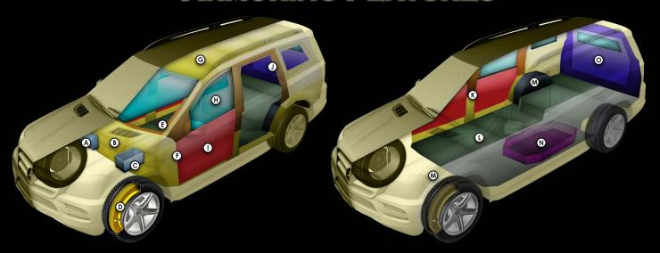
\*\* These schematics represent typical armoring of an SUV. The final vehicle (IFFP GRAND CHEROKEE LIMITED) may vary depending on the client's required specifications.
