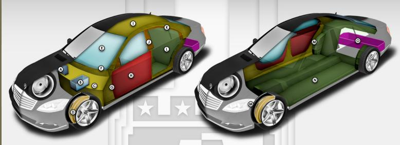
\*\* These schematics represent typical armoring of a truck. The final vehicle (Hyundai Genesis G90) may vary depending on the client's required specifications. \*\*
