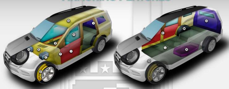
\*\* These schematics represent typical armoring of an SUV. The final vehicle (Ford F-350 Super Duty) may vary depending on the client's required specifications. \*\*
