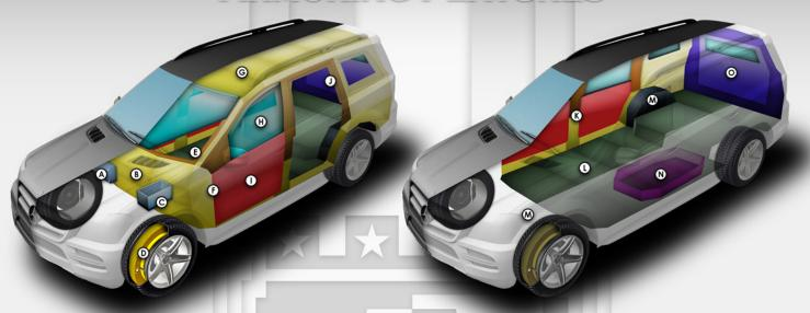
\*\* These schematics represent typical armoring of an SUV. The final vehicle (Hummer H1 Alpha) may vary depending on the client's required specifications. \*\*
