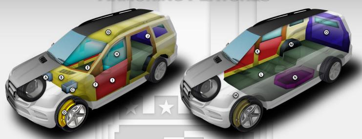
\*\* These schematics represent typical armoring of an SUV. The final vehicle (JEEP Grand Cherokee Limited) may vary depending on the client's required specifications. \*\*
