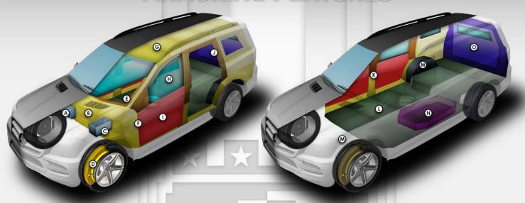
\*\* These schematics represent typical armoring of an SUV. The final vehicle (Cadillac Escalade) may vary depending on the client's required specifications. \*\*
