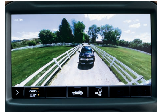
Rear Trailer View Uses an available accessory camera that can be installed to show vehicles or objects behind the trailer.
