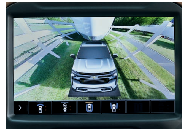
Bowl View Provides a rear-facing 3-D surround view, useful for low-speed backing maneuvers.
